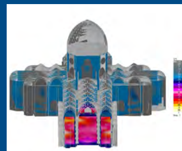
EASE Simulation: STI index prediction with two Ascolto LH6425 over listening area (church nave)
