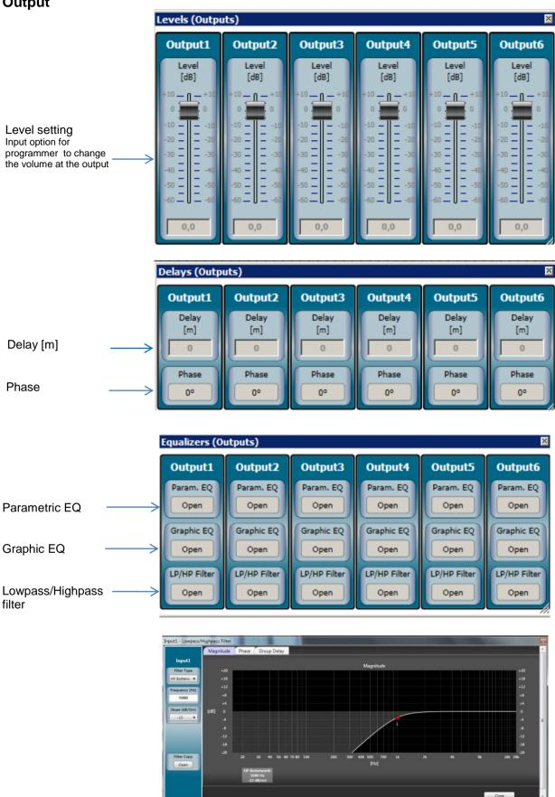
Each output has a 31 band graphic equalizer. All parameters can be copied to the other EQs or individually adjusted for each output.
