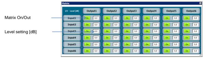
After pressing the right mouse bottom a pull-down menu opens. It allows the activation of all matrix nodes or different rows or columns of nodes. Routing of all inputs and outputs with additional level setting.
