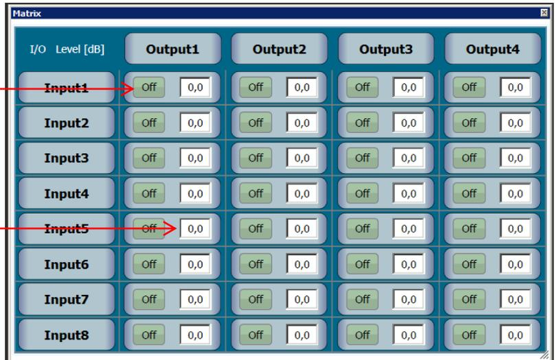
After pressing the right mouse button a pull-down menu opens. It allows the activation of all matrix nodes or different rows or columns of nodes. Routing of all inputs and outputs with additional level setting.
