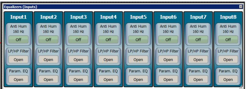
8 parameters are available for each input and each output. The settings can be copied to each other input and output. The same applies to the highpass/lowpass filters.
